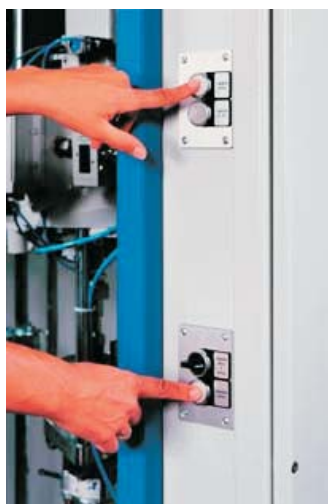
Two-hand control for drum change
