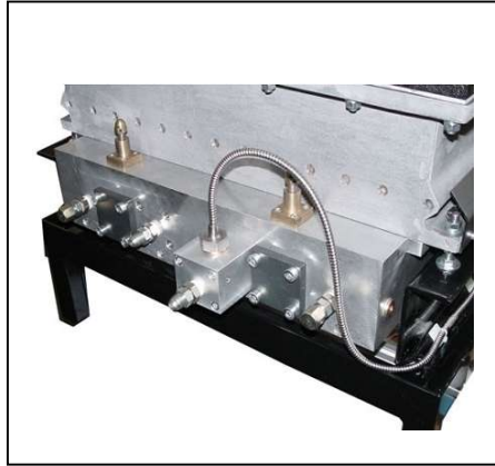
Pressure measurement at filter block
