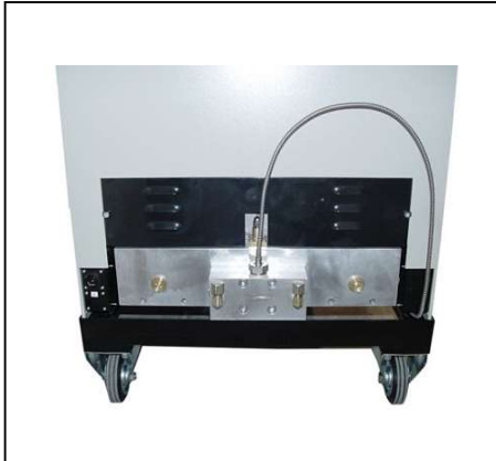
Filter block with pressure measurement
