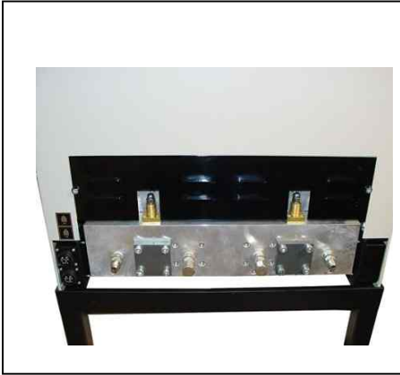
Two pump unit with bypass
