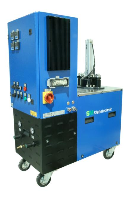
Bag melter for processing 2 Kg PUR-peelable bags
