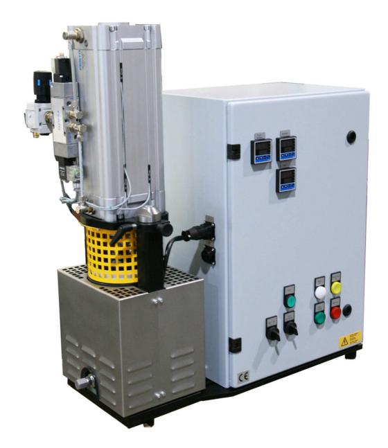
for the gentle melting from 2 kg PUR candles within foil bags Ø127mm. Without pump and Bypass usage. With adjustable adhesive pressure from 1-6 bar. The unit is working by " melt on demand " principle.
